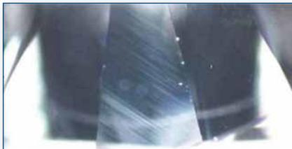
The picture shows an image of polishing lines on a pavilion half. Heavy polishing lines are clearly visible as a pattern of white stripes under oblique light. The polish grade will depend on the visibility of the polishing lines.
