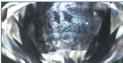
Burn marks look like faint oil stains on the facet. These marks can be more obvious when looking at the defect through the diamond from the opposite side. The cause of burn marks is oxidation of the surface due to overheating the diamond during the polishing process.
