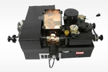
A Parallel axis bruting machine (Maxi cut) for first/second bruting
