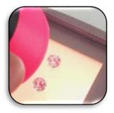
Sit the diamond in one of the two holes. Place the calibration CZ in the other hole.
